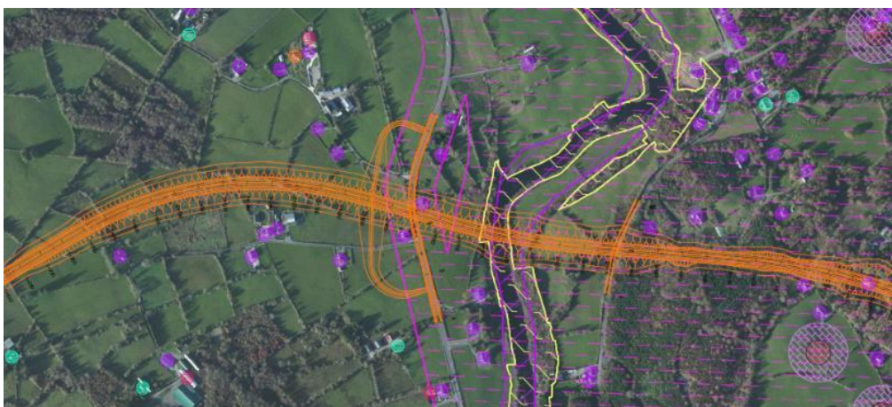
FIGURE 2.2: COMPACT GRADE SEPARATED JUNCTION WITH R252
